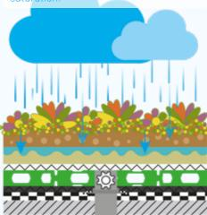
When fully saturated, the ND WSM-50 Water Reservoir Panel buffers 40 l/m<sup>2</sup>
