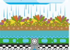
After the rain has stopped the water retained in the ND WSE-100lte Water Retention Element, continues to flow at the set flow rate into the storm water system.
