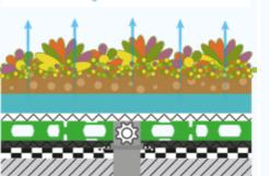
Depending on the intensity and frequency of rainfalls, the main amount of the water will be retained in the vegetation layer and ND WSM-50 Water Reservoir Panel. Only during extreme rainfall, the ND WSE-100lte Water Retention Element will have a retention function. Generally, the water fully contributes to the evaporation and transpiration, enhancing the small water cycles by returning the water to its
