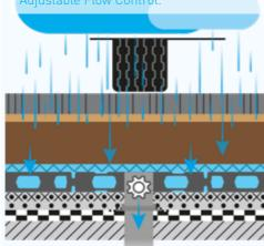
After the rain has stopped the water retained in the ND WSE-80hd Water Retention Element, continues to flow into the storm water system at the set
