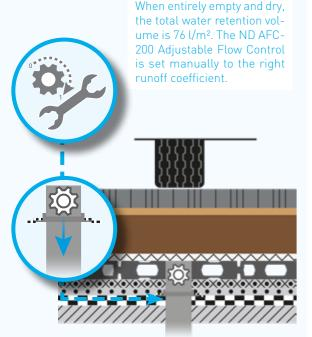
Rain shower occurs and the rain flows through the laying course and subbase layer into the ND WSE-80hd Water Retention Element with a retention volume of 76 l/m<sup>2</sup>. The water is stored here temporarily for a period that is set by the culated flow rate of the ND AFC-200 ustable Flow Contro
